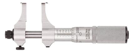
Figure 2.16.4: Inside of the Micrometer
