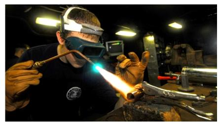
Figure 2.7.6: Oxyfuel gas welding
