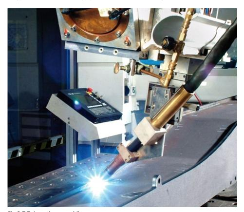
Fig 2.7.7: Laser beam welding
