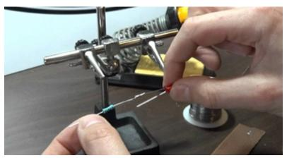
Fig 2.15.1: weld the copper lead wire to resistor
