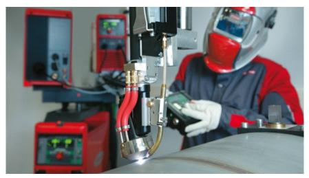
Figure 2.7.5: Plasma arc welding
