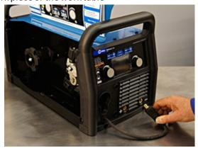
Fig 2.3.10: connection of the work clamp
