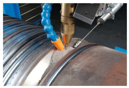
Figure 2.7.2: Submerged arc welding
