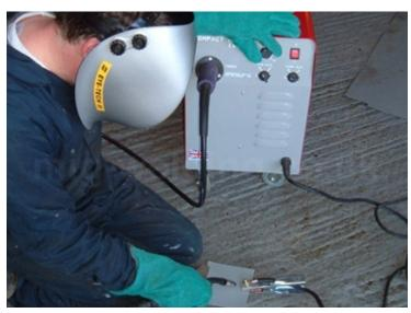
Fig 2.3.17: checking the setting of the speed of the wire feed
