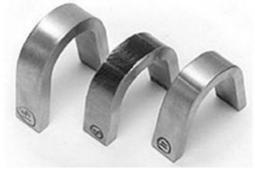
Fig 2.11.2: bend test coupons for the welding procedure qualification
