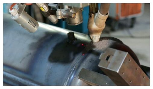
Fig 2.7.3: Flux core arc welding (FCAW)
