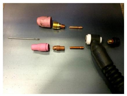
Fig 2.3.14: assembling the torch
